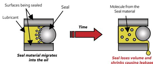
**Seal swell** – lubricant components migrate into the seal matrix. Moderate seal swell is welcomed whilst over swelling can cause deformation and leakage.
