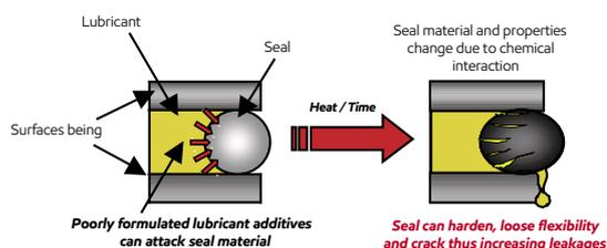
Many other environmental aspects can impact the seal's performance, such as higher temperatures that can accelerate chemical reaction, and dust/dirt and other contaminants that can cause seal wear. It is very important therefore that the lubricant and seal are as compatible as possible to optimize the system's efficiency.
