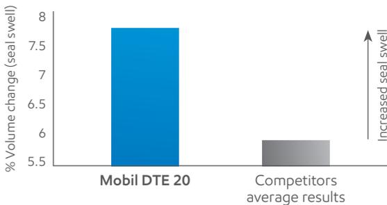
Mobil DTE 20 is designed to provide extra seal swell properties as demonstrated by the results of this test. This higher swell tendency, which is within manufacturers guidelines, can help reduce oil leakage resulting from oil/seal interactions.
